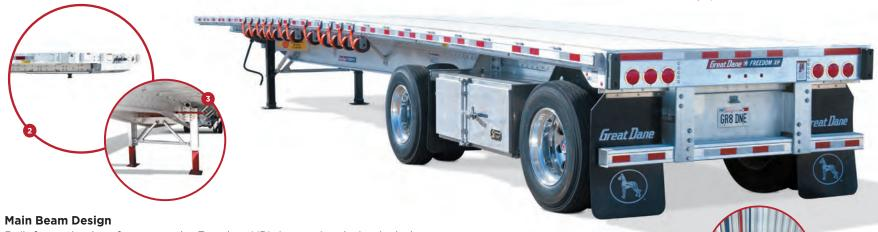
Built for optimal performance, the Freedom XP's innovative design includes a two-piece riveted main beam that is contoured for optimal swing clearance and engineered to deliver superior strength. Multiple beam configurations allow for concentrated load ratings from 52,000-60,000 pounds and evenly distributed load ratings from 80.000-120.000 pounds.
