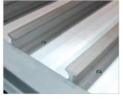
Long Life Floor System Great Dane's reefer cargo and heavyduty Safety Grip duct floors are automatically welded to seal out moisture. Composite sills support the floor continuously for maximum support and are anchored by corrosionresistant sill screws. An impact-resistant thermoplastic sub-pan completes the floor design for maximum durability.
