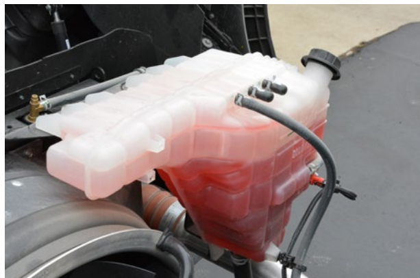
Translucent containers allow you to check fluid levels at a glance.
